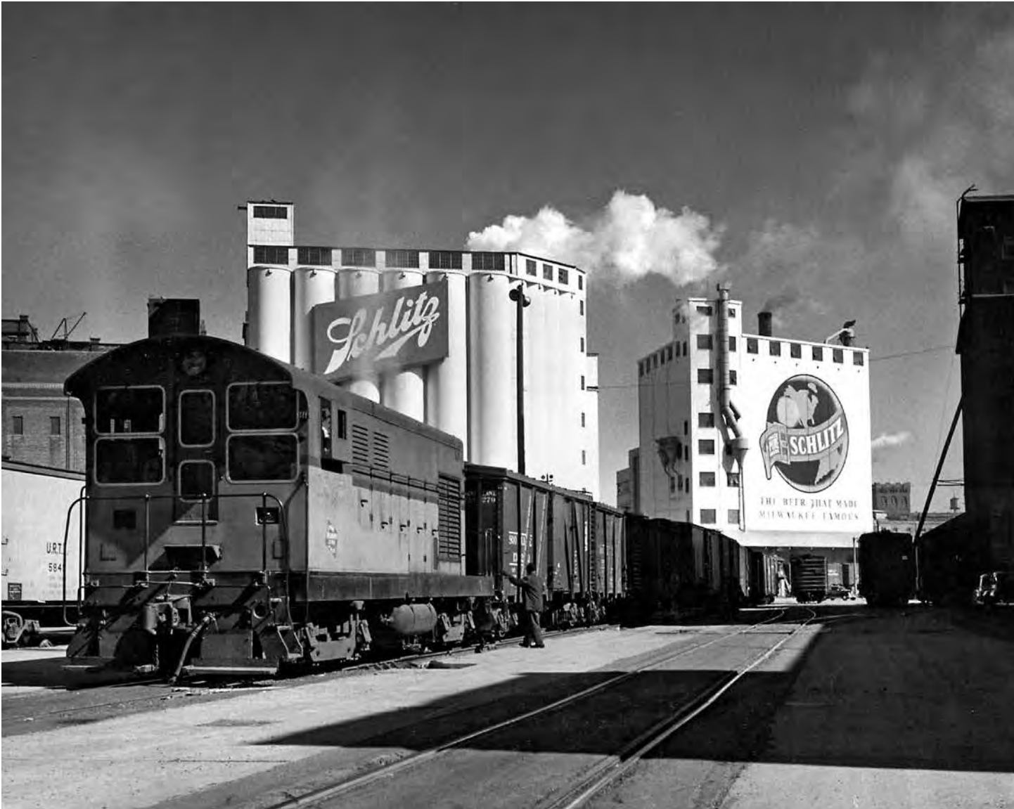
Milwaukee Road Fairbanks-Morse locomotive switching boxcars at the Schlitz brewery on the "Beer Line" in Milwaukee, Wisconsin, in 1952. Photograph by Wallace W. Abbey, collection of the Center
