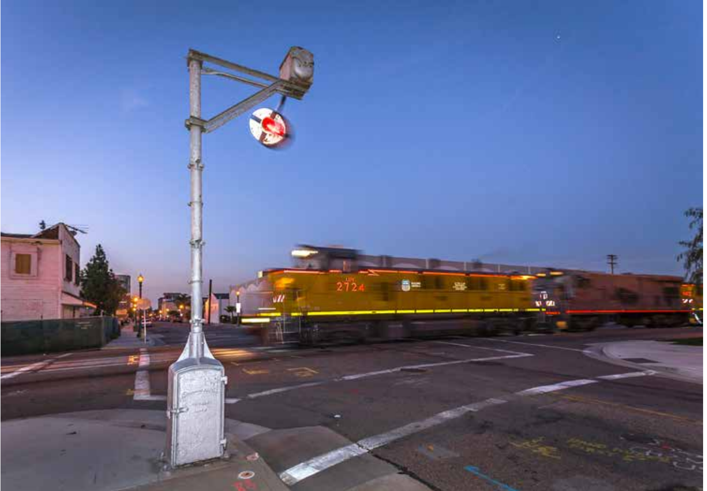
Above: Union Pacific's "Marlboro Local" passes a wig-wag crossing signal in Anaheim, California, in 2008. Photograph by David Styffe
