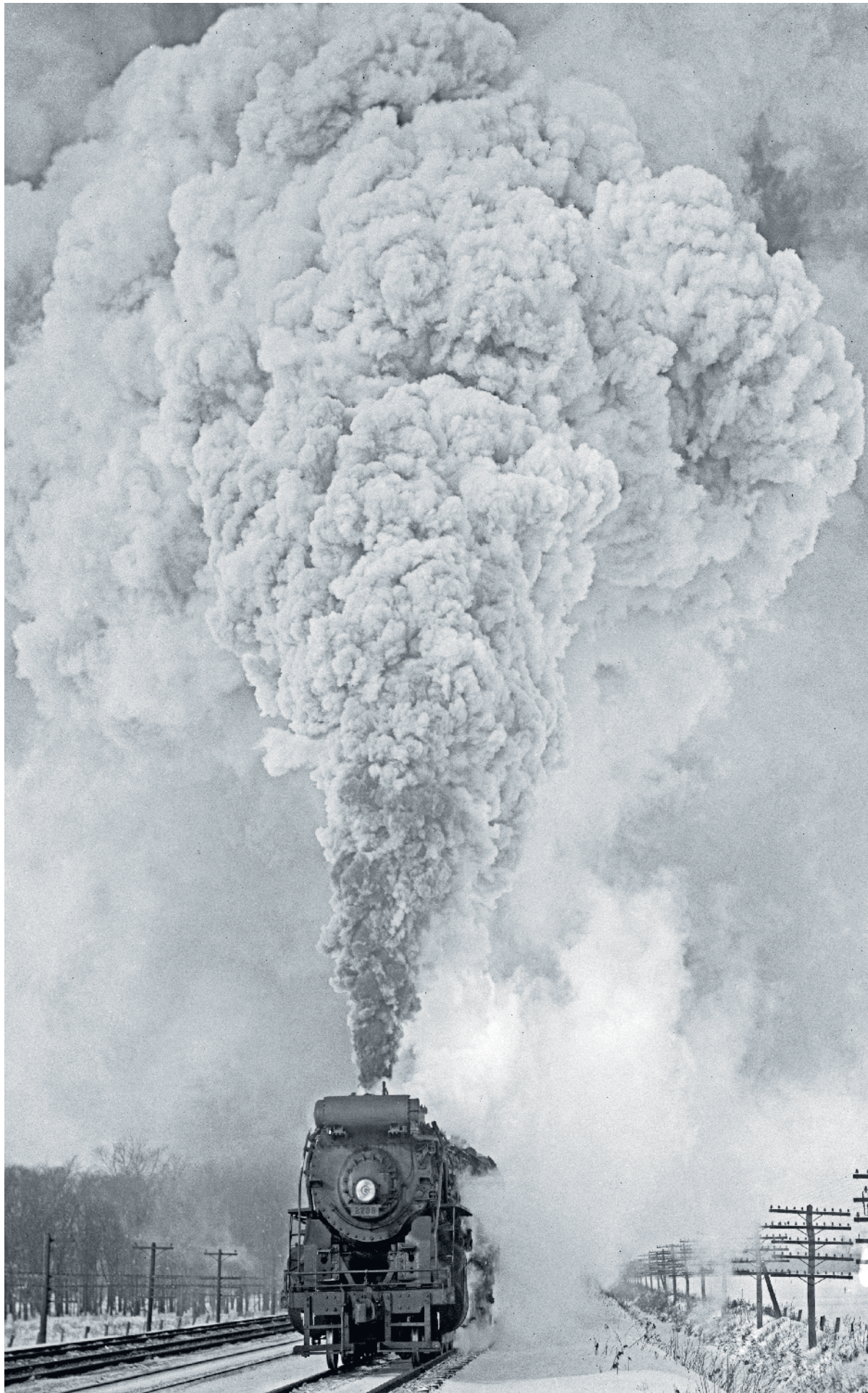
Left: New York Central Railroad L-2a class 4-8-2 steam locomotive no. 2739 sends an eruption of steam and smoke into the winter sky as it powers a train down the railroad's four-track main line sometime around 1950. Photograph by Robert A. Witbeck. Witbeck-02-020-04
